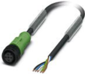
Sensor/Actuator cable, 5-position, PUR halogen-free, Black-gray RAL 7021, Free cable end, on Socket straight M12, A-coded, Cable length: 3 m, with plastic knurl
